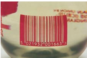
Fig. 10, Bad colors and deformed barcode due to bottle curvature.
