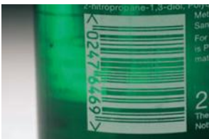
Fig. 11, Bottle substrate and color used as bars in the barcode.
