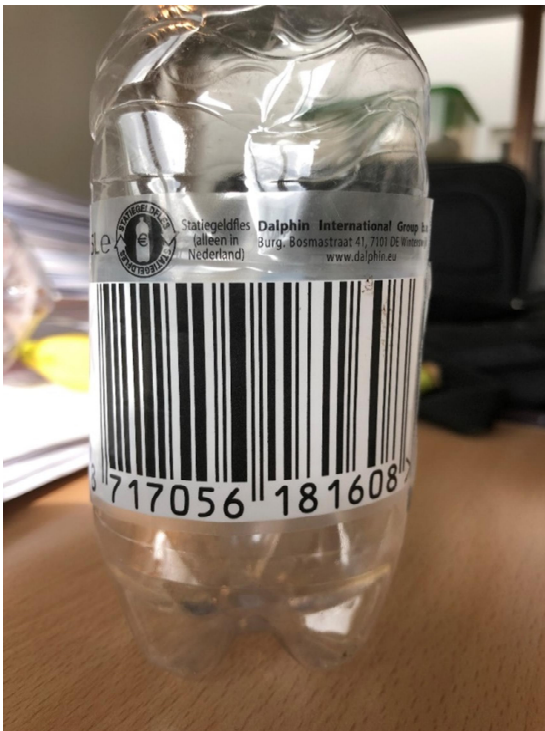
Fig. 4, Picket fence barcode wrapped around a PET bottle.
