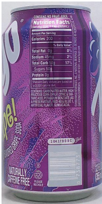
Fig. 12, Barcode printed with white bars on the raw metal surface giving a bad contrast.
